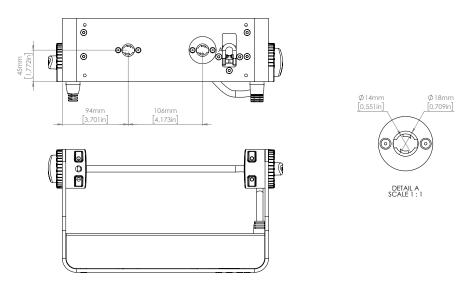
Figure 3: Dimensions for Q-2 base locking points
