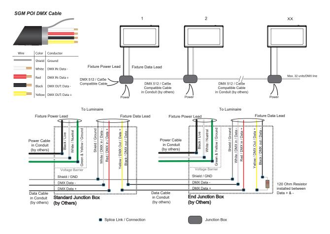
Figure 19: Connecting DMX and AC Power in Q-2 POI
